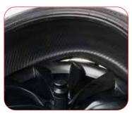
Quick demounting procedure with bead breaker disc. Quick procedure for demounting the lower bead (particularly suitable for hard sides).
